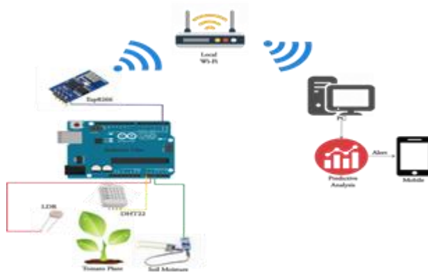
Figure 2: IoT based Watering System
