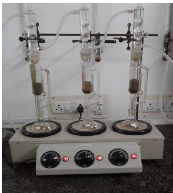
Fig.1: Soxhlet apparatus used in the present work
