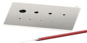
Figure 3 Neuromuscular Steadiness Tester
